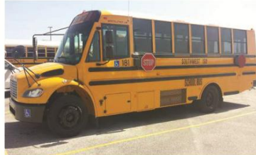
Thomas School Bus with Cummins 6.7 turbo diesel engine using the ECO-4
