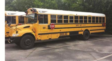
International School Bus with a DT-466 International inline 6 turbo diesel engine - ECO-4
